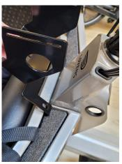
2.1 Place the Lockride with the two small hooks between the foam and the top tube.
