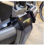
**3.3** Mount the slide in the bracket and attach the Abus Diskus lock.
