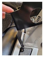
2.2 Tilt the lock vertically and now press the battery lock down along the top tube with considerable force. The foam will be pressed in slightly, but it will bounce back later. To prevent damage to the top tube, you can also use 2 plastic cards in the places between the top tube and the 2 hooks to guide the battery lock in the downward movement.
