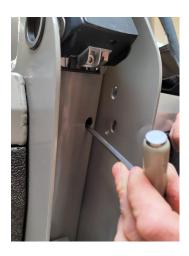
**1.1** Remove the battery from the bicycle and slightly loosen the 2 Allen screws under the battery (maximum 3 rotations).
