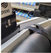
**3.1** Retighten the 2 bolts under the battery.
